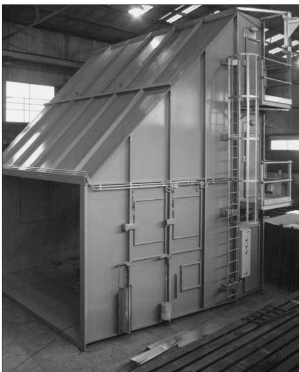
Gas turbine air intake housing for 515000 m 3 /h
